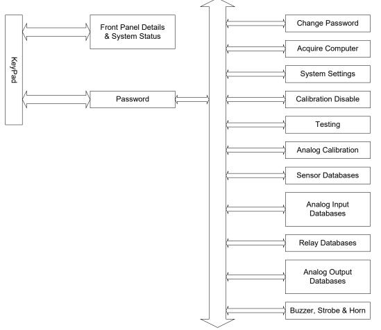
Note that while in the Menu Tree, all normal monitoring operations stop. The alarm status does not change.
